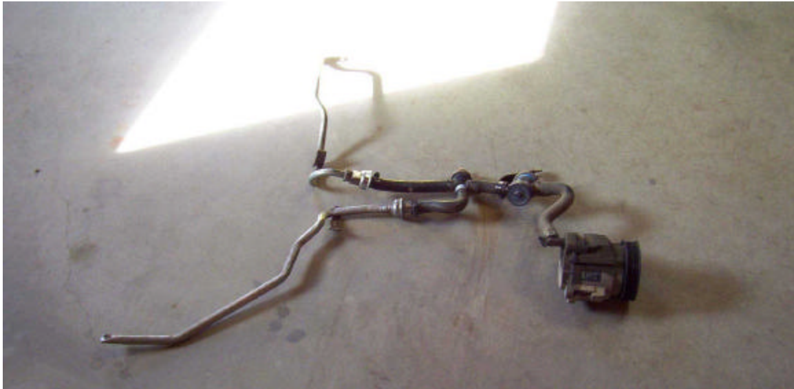
Figure 12. Here it is. You can see how my tube that goes to the exhaust under the car was already cut off, crimped and welded shut. I just had to break the tack weld that held it to the exhaust. Normally this would need to be cut off and the hole in the exhaust welded shut.
