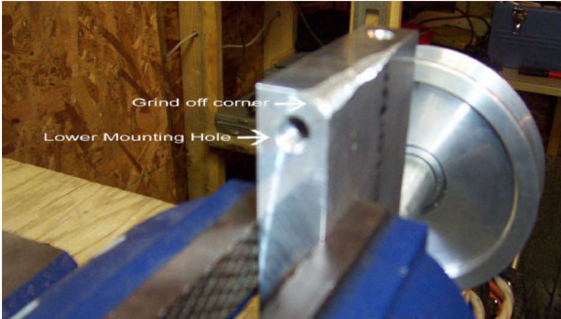
Figure 17. Showing the removed corner from mounting block. I used a side grinder but this could be accomplished with a file as well.
