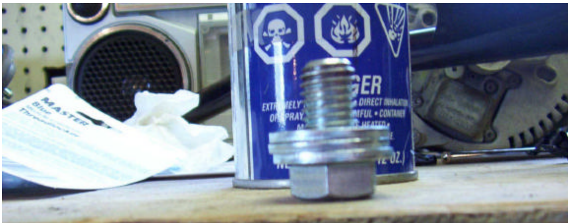
Figure 13. Here you can see the bolt used to plug the holes in the heads with the three washers installed. Bolt – \frac{9}{16} " NC GR5.
