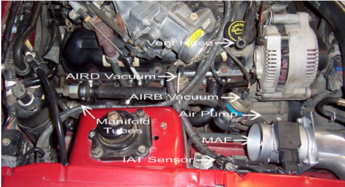
Figure 2. Air inlet tube removed. Unplug the Vent hose and IAT sensor from the inlet tube and loosen the clamps at either end and remove the inlet tube. You can now clearly see the AIRB (Bypass) and AIRD (Diverter) valves and most of the associated hoses that will be removed.
