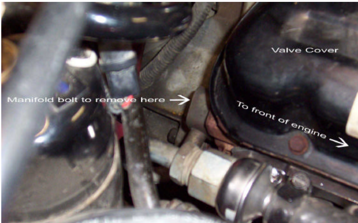
Figure 5. Shows the passenger side location of manifold tube bolt to be removed. This looks to be the easy side but it wasn't.
