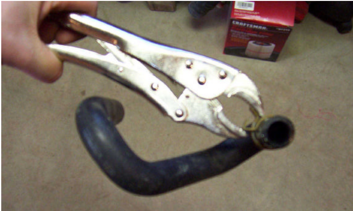
Figure 16. Use a vise grip so you don't have to try to hold the clamps open. These clamps require quite a bit of force to hold open.
