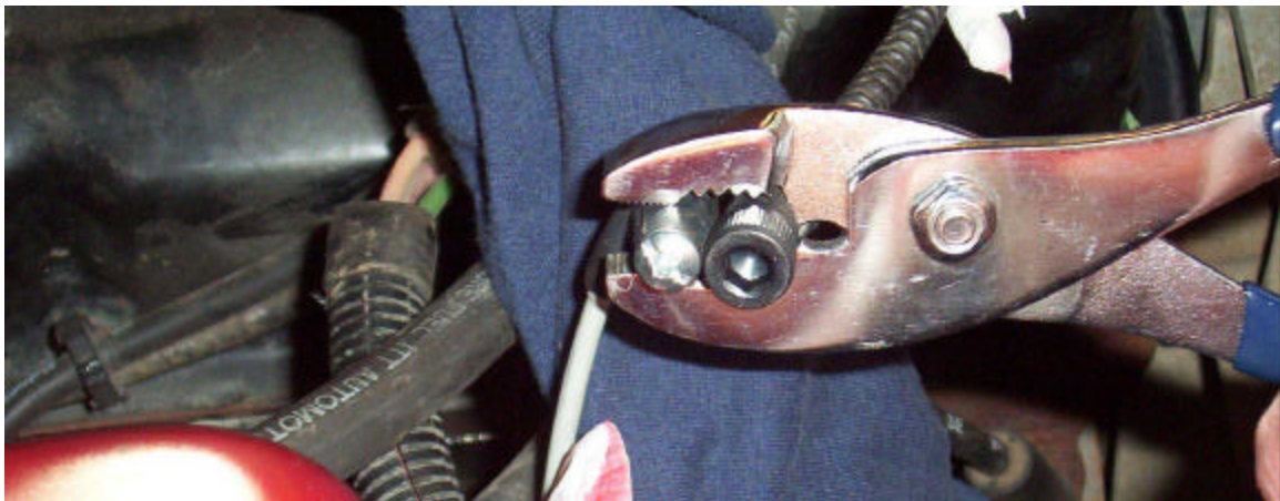
Figure 15. Showing the vacuum lines plugged. The bolts or screws should be large enough to require a screwdriver to turn them in, this will ensure a positive seal.
