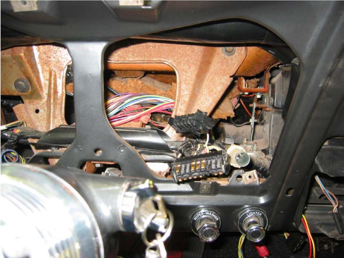
Before reinstalling the terminals into the new plug, be sure to **bend the tab back out** (**bend down**) so that it clicks when the metal terminal is fully pushed into the plug. Give a slight tug on the wire to make sure it won't come back out.
